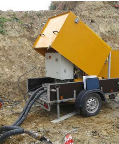
GROUND RESPONSE TEST - ASTI (BN) 50kW
